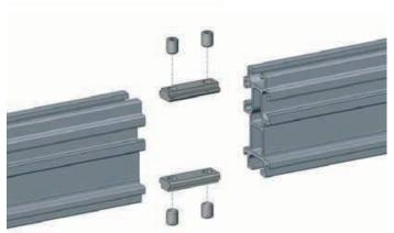
The coupling set C75 is used as connecting element for the rail profiles C75. The sliding block spare positioned in the upper and lower groove on the rail profile and secured with the aid of setscrews. The cup points of the setscrews generate the required tight fit. With the aid of the couplings et the rail profiles can be connected to any length offline.
