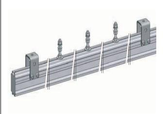
Two different fastening components are available so that the longitudinal extension of the rail line caused by temperature changes is no to be strutted. The fixed point mounting is only used once per rail line, preferably at the start of the rail. it fixes the rail in all three planes. The Sliding Hanger used at all other suspension points and ensure problem free longitudinal extension of the rail line. The distance between hangers on the rail is 2 to 3 m depending on the load situation.
